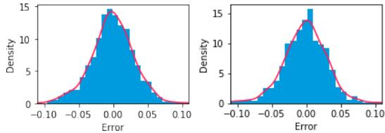
**Fig. 1.** Density plots for the errors for the entropy (left) and regularity (right) FIN reconstructions. The feature values were scaled and normalized, making the biggest possible error 1, as can be observed the FINs faithfully recreate the closed form equations.
